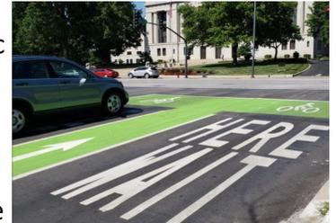
**Queue Box:** Also known as a two-stage turn box, this is a space that offers bicyclists a safe way to make left turns from a right side bike lane. Bikes can use the box to reposition and wait until a traffic signal turns green at a signalized intersection, or until traffic is cleared at an intersection without a signal. Drivers should not park or stop in the queue box.
